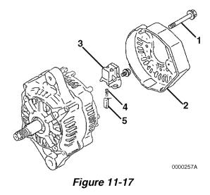
10. Reinstall the rear cover (Figure 11-17, (2)) to the rear frame housing with three bolts (Figure 11-17, (1)).
