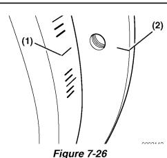
Highlight the target timing mark (Figure 7-26, (1)), (Figure 7-27, (1)) on the flywheel timing grid as determined in the *Fuel Injection Timing Chart* below.
