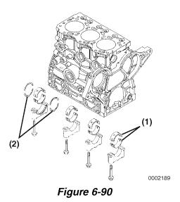
3. Install the crankshaft in the engine.
