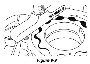
Record the measurement. *See Outer Rotor Side Clearance on page 9-4 for the service limit.*
