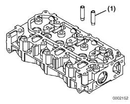
Finish installing the valve guides
