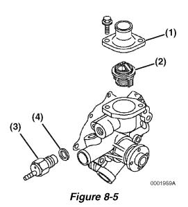
Remove the thermostat (Figure 8-5, (2)). Remove the temperature switch (Figure 8-5, (3)) and gasket (Figure 8-5, (4)). Discard the gasket.
