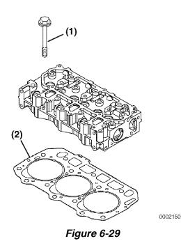
Lightly oil the threads of the cylinder head bolts (Figure 6-29, (1)). Tighten the bolts to the specified torque shown in the chart below. Tighten in the sequence shown in Figure 6-30. See Torque for Bolts and Nuts on page 6-13.
