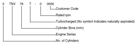
When ordering parts or making an inquiry about the engine you are working on, be sure to include the complete model and serial numbers as shown on the engine nameplate. *See Location of Labels on page 4-4.*
