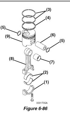
Note: Reinstall the top and second piston rings with the stamped "makers mark" (Figure 6-87, (1)) facing the top of the piston. The "makers mark" may vary in appearance but will always be located on the top surface of the piston ring adjacent to the piston ring gap. The oil ring and oil ring expander can be installed either side up.
